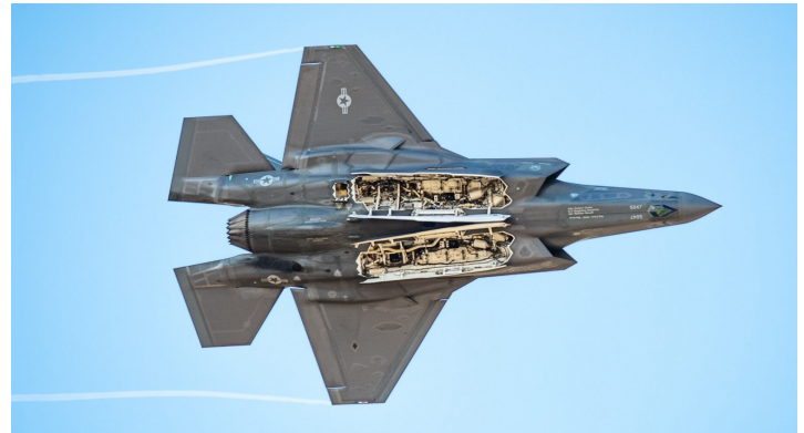
An F-35A shows off its internal weapons bays.
